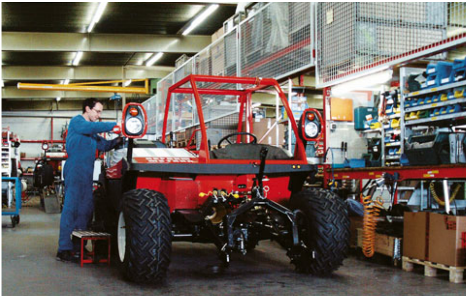
A “Metrac” nears completion: The platform concept is the basis for meeting specific client wishes at the same time as manufacturing economically.
